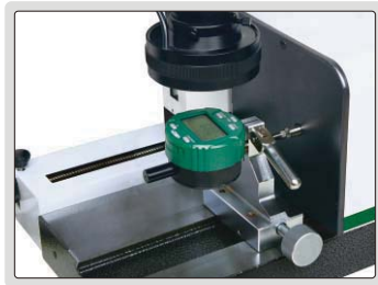
check digital indicators (detect digits on screen)
