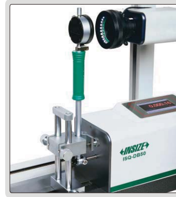
check bore gages
