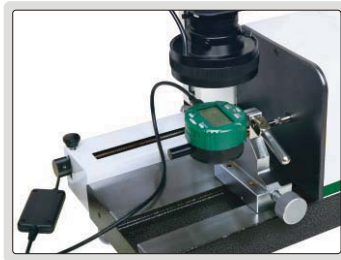
check INSIZE digital indicators (connection with cable)
